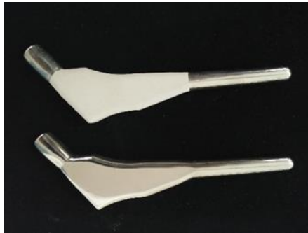
Figure 5: The final product, uncoated and coated with HA powder
